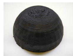
Figure 2: Simple hemispherical anatomically accurate breast phantom created using heterogenous mixture of the two tissues.
