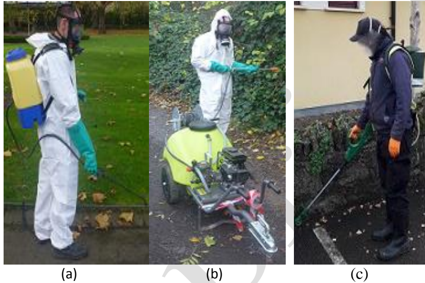
Figure 1: (a) Manual Knapsack sprayer with a handheld manual lever (b) Pressurised lance is a motorised portable applicator with a handheld lance (2-3 bar pressure) (c) Controlled droplet applicator with adjustable droplet size and pre-mixed solution.
