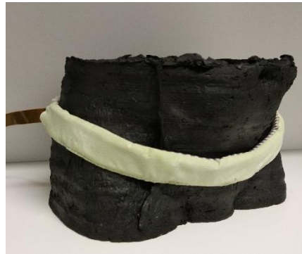
Figure 6: Illustration of the Swisstom electrode belt fitting on the phantom. The belt is 44 cm long and consists of 32 electrodes. Ultrasound gel was used between the electrodes and pelvic phantom to improve the contact impedance.
