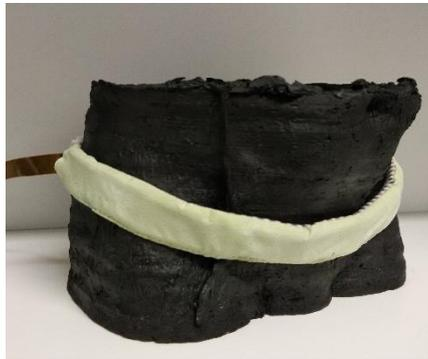
**Figure 6:** Illustration of the Swisstom electrode belt fitting on the phantom. The belt is 44 cm long and consists of 32 electrodes. Ultrasound gel was used between the electrodes and pelvic phantom to improve the contact impedance.
