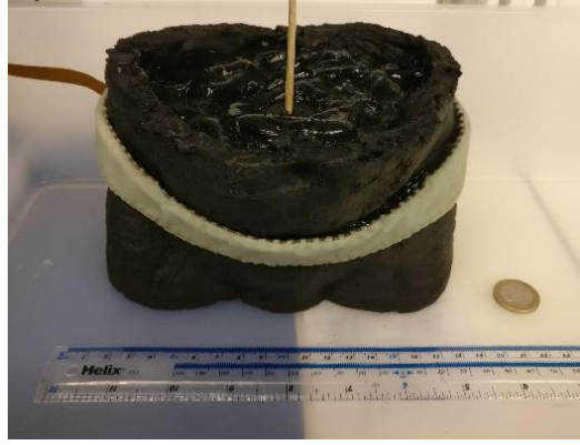
Figure 2. Phantom experimental setup. The bladder is submerged in ultrasound gel within the anterior region of the phantom. Further details on the experimental setup are available in Dunne et al. 22 .
