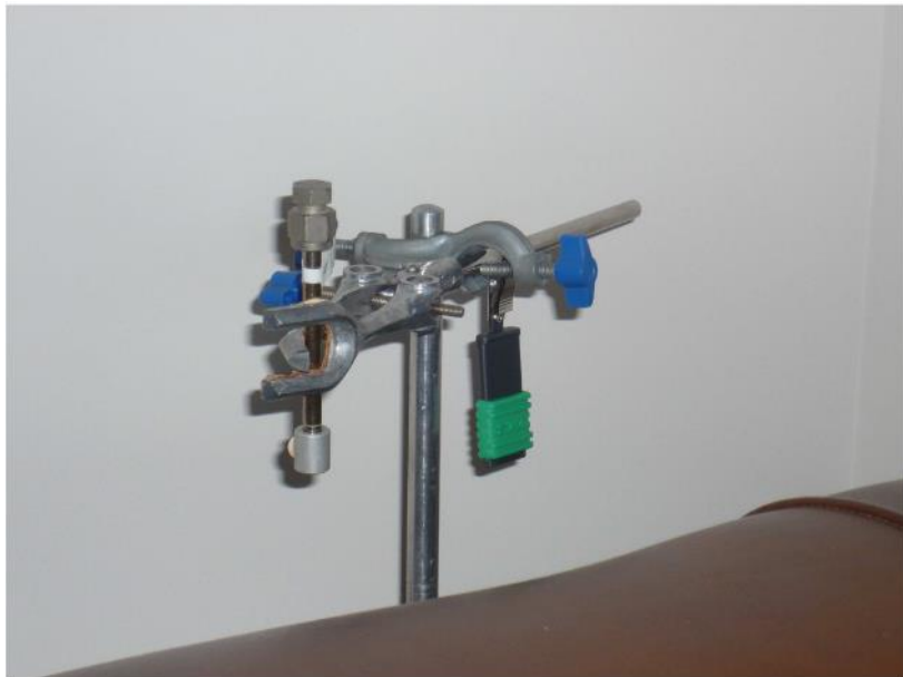
Picture 2: Passive Sampling of Formaldehyde (black and green badge) and TVOC's (metal tube).
