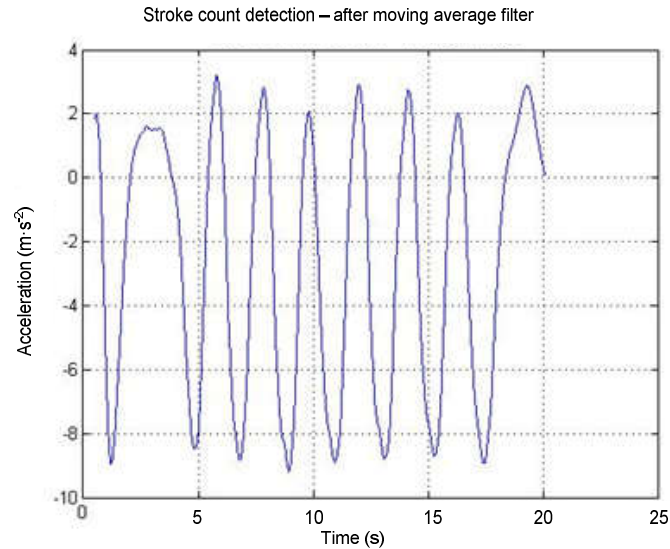
Figure 8.36. The detection of each peak in the X-axis acceleration signal for stroke count determination is made easier by using a moving average filter over a 0.5 s window to smooth out the signal.
