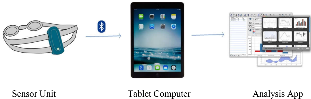
Figure 6.4. Description of the swimming sensor device system components.
