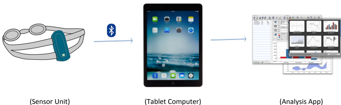
Figure 2: Description of the swimming sensor device system components.
