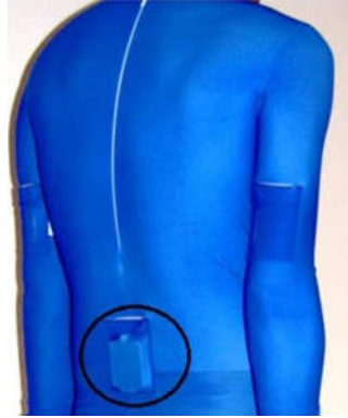
Figure 4.19. A modified swim suit design allows for accurate positioning of the sensor device but may result in unwanted sensor movement. Reproduced with permissions from Dadashi, et al. [97].
