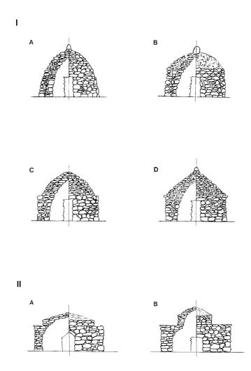
As visible from the typology and the attached drawings, there are two types of construction in evidence. However, it is also necessary to pay attention to some differences in the design and the static construction of the door. Namely, along with the obvious difference in the ground-plan disposition there are also two designs of the entrance space:
