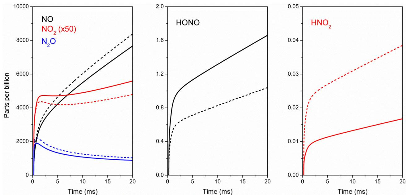
**Figure 2.** Effects of updating thermochemical values within a literature model<sup>16</sup> on the prediction of several important nitrogenous compounds under typical gas turbine operating conditions. Dashed lines refer to results using the original model, while solid lines correspond to the updated model.
