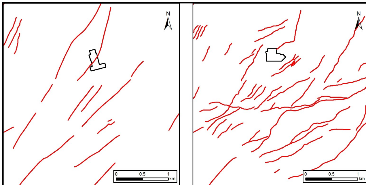
Figure 5. The impact of fault mapping on the final location of the Te Mihi Power Plant. Left: location of known active faults prior to this study and initial proposed site of the Te Mihi Power Plant. Right: location of active faults mapped in this study and the subsequent location of the Te Mihi Power Plant.
