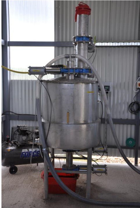
Figure 6-1 Meso-scale reactor used in this experiment
