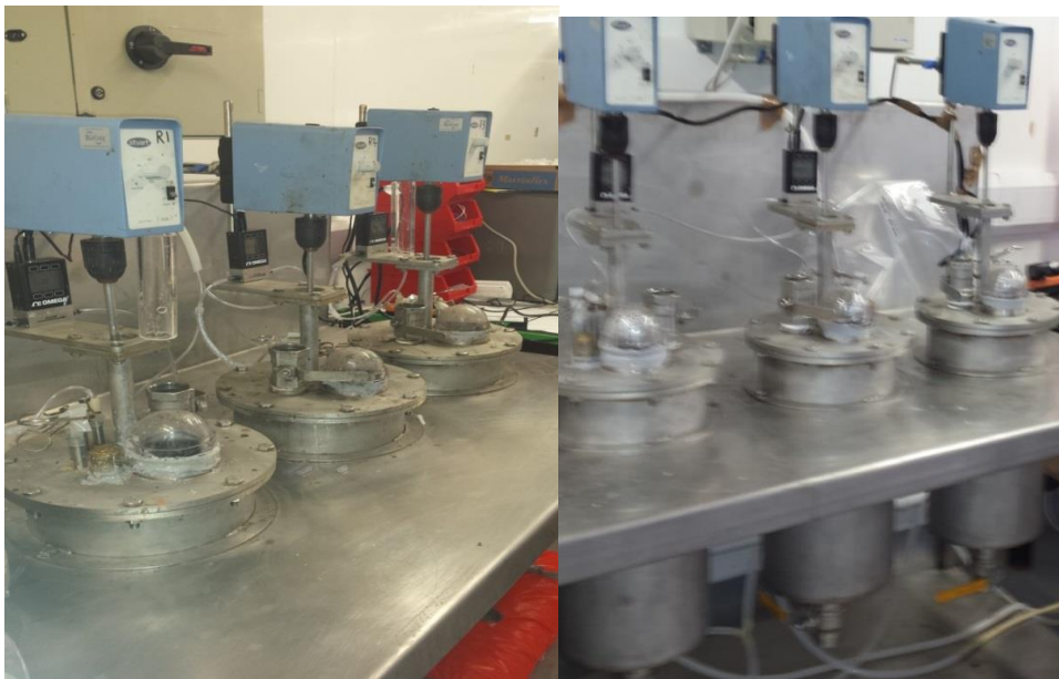
Figure 4-1 The semi-continuously stirred reactors used during the study
