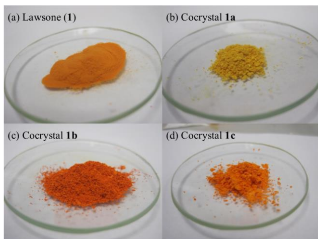
Fig. 3 Photographs of Lawsonsone ( 1 ; a) and the cocrystals synthesised using 4,4'-bipyridine ( 1a ; b), 4-(2-pyridine-4-ethyl)pyridine ( 1b ; c) and 1,3-di(4-pyridyl)propane ( 1c ; d), illustrating the observed colour changes.
