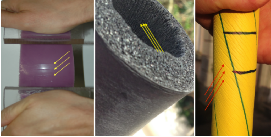
Figure 1: Creases appearing in the large deformation of soft matter, as indicated by arrows. Left: Large bending of a silicone block with two ends glued to plastic plates, on which bending moments are applied; Middle: Everted tube of pipe insulation material; Right: Twisted cylinder, on which axial and circumferential lines were drawn prior to the twist. Notice how all creases are aligned with a principal direction of stretch.
