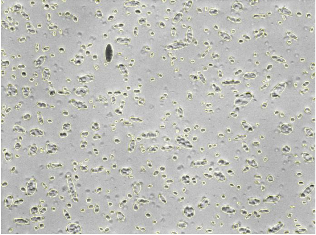
Fig. 6.8: Snapshot highlighting the detected particles and their approximate sizes. The black smudge is a RBC being sheared at \tau = 7 Pa .
