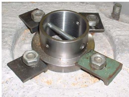
**Fig. 3:** Pile-to-raft fixity arrangement
