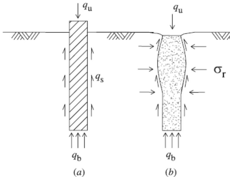
Figure 3: Mechanisms of load transfer for (a) a rigid pile and (b) a stone column (after Hughes and Withers 1974)
