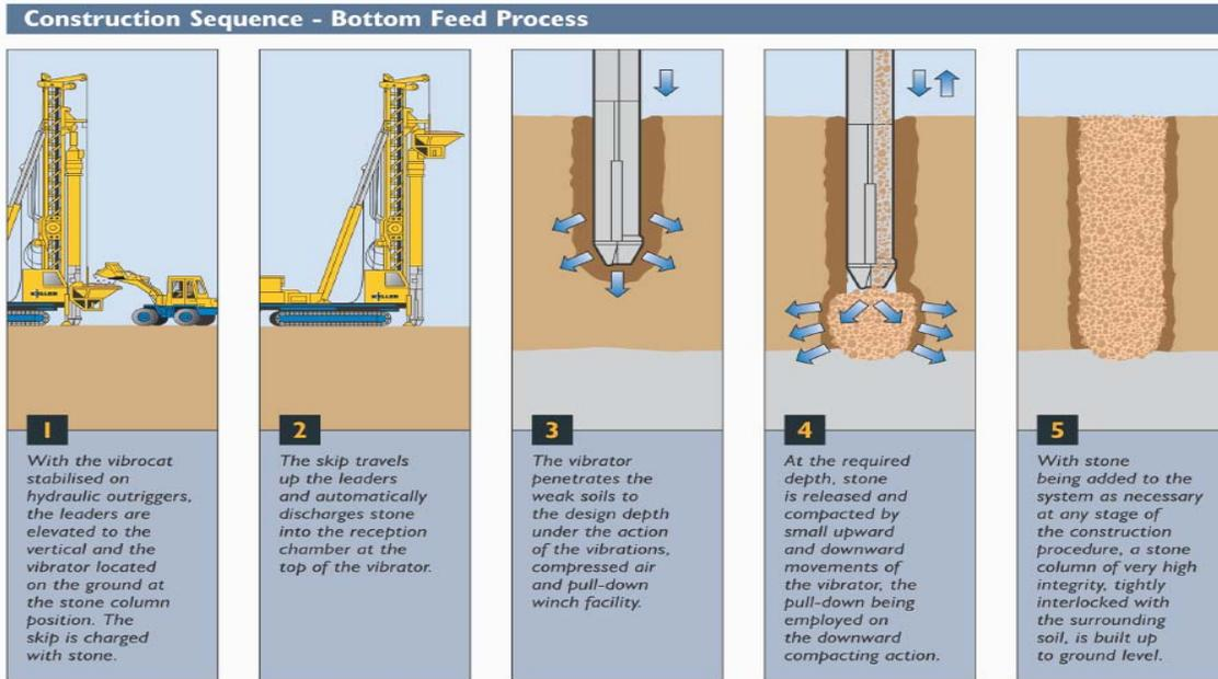
Figure 2: Bottom Feed method of stone column construction
