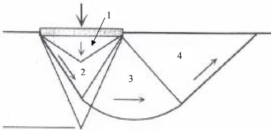
Figure 7: Four-zone failure mechanism proposed by Muir Wood *et al* (2000) for stone column groups
