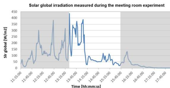
Figure 10. Solar global irradiation measured during the experiment on January 27<sup>th</sup>, 2014.
