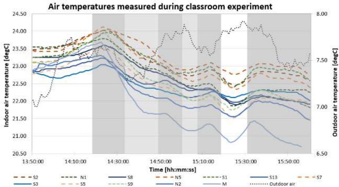
Figure 7. Air temperatures measured during the experiment on February 13<sup>th</sup>, 2014.
