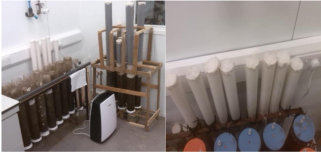
Figure 3.5 - (a) Laboratory setup for Experiment A (b) Surcharged small specimens behind rack and columns with lids for gas sampling
