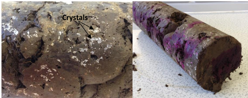
Figure 5.1 - (a) Crystals on P3(3) (b) P3(3) after phenolphthalein indicator application
