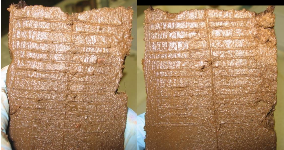
Figure 3.14 - Stabilised peat specimens with 5 mm depth intervals lined out for (a) b3(2c) and (b) b8(3c)
