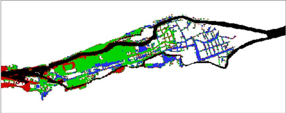
Figure 12. Map of fluvial inundation due to maximum river flow of 300\text{m}^3/\text{s} (red), 500\text{m}^3/\text{s} (green) and 700\text{m}^3/\text{s} (blue)
