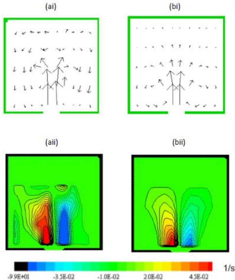
Figure 2. Flow pattern in the harbour: observations (a), and  $k-\epsilon$  model (b), velocity (i) and vorticity (ii). Model simulated velocity and vorticity mapped on the observational grid for comparative purposes
