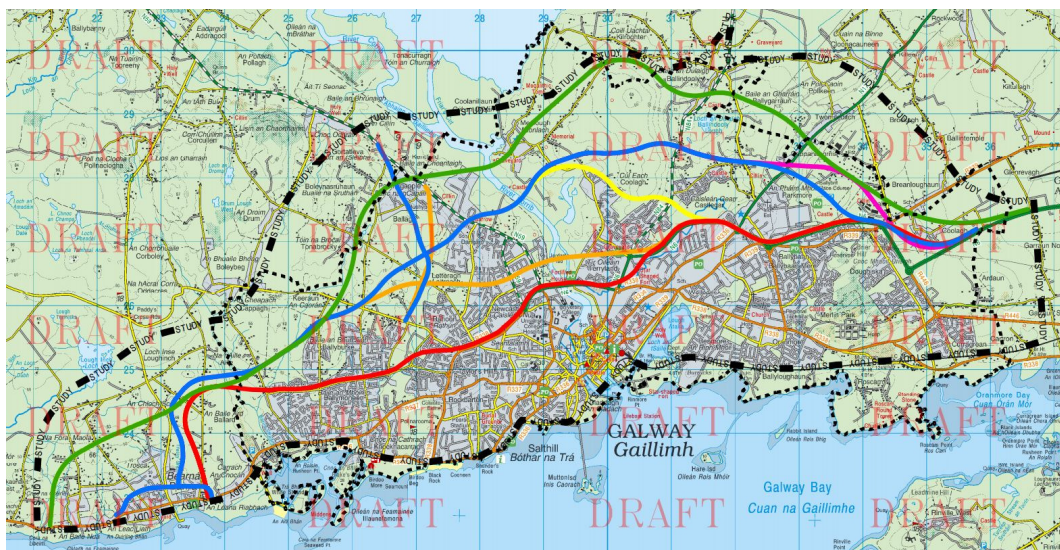
Figure 2.11 - N6 Transport Project route options (ARUP, 2015)
