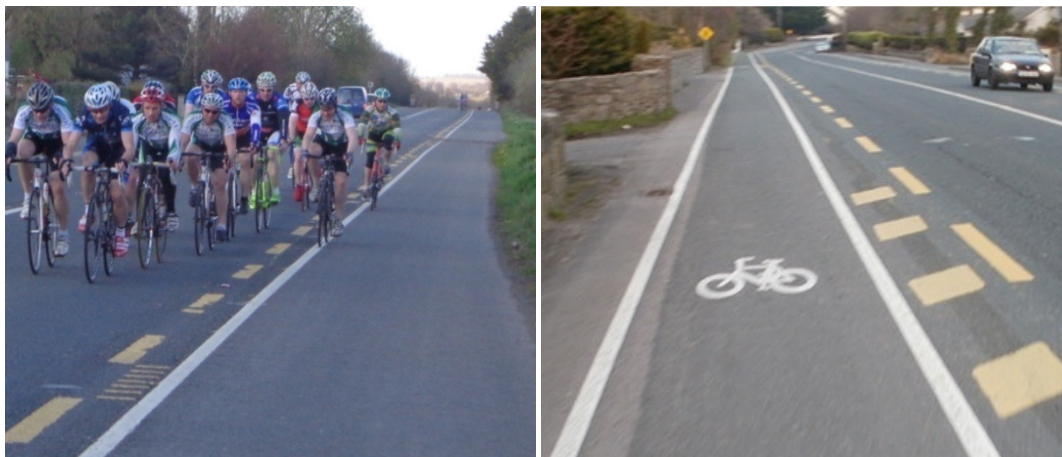
Figure 8.7 - On-road cycleways R445 Limerick to Nenagh (Limerick Cycling Club, 2013) (left) and R292 Sligo to Strandhill (ROD, 2013) (right)
