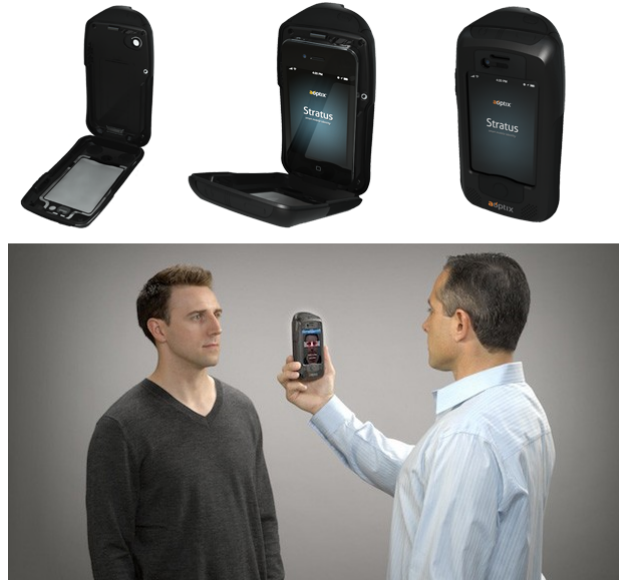
Fig. 2.15 AOptix Stratus - the iPhone wrap-around device for biometrics. A use case scenario is also shown. Adapted from [72].
