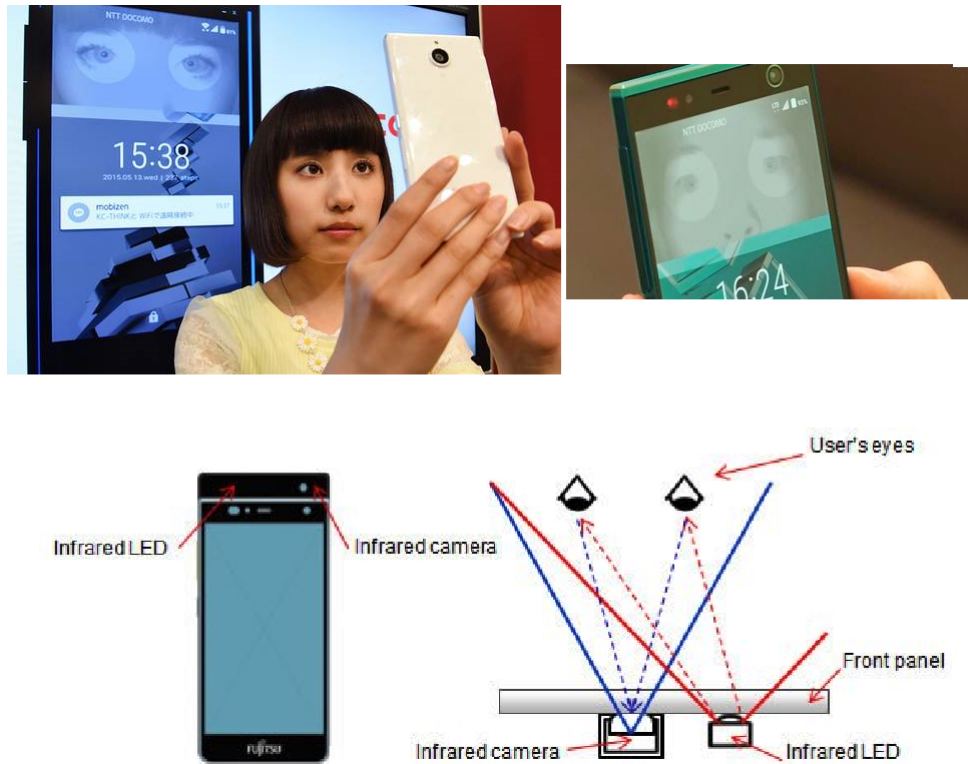
Fig. 2.16 NTT DoCoMo - Fujitsu ARROW NX F-04G: World's first smartphone with iris recognition. An additional infrared LED and infrared camera is used for iris recognition. Eye bands are provided for eye alignment. Adapted from [33, 74].
