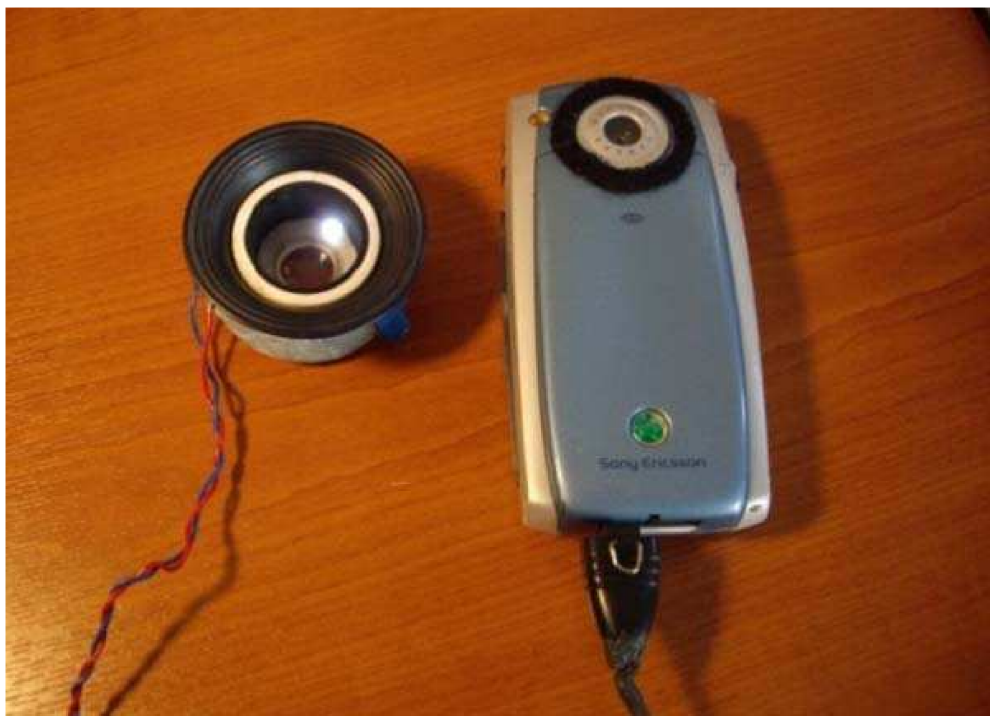
Fig. 2.14 ‘Eye cup’ with a luminous diode attached to a Sony Ericsson P800 to capture iris images with uniform illumination and stand-off distance [71].
