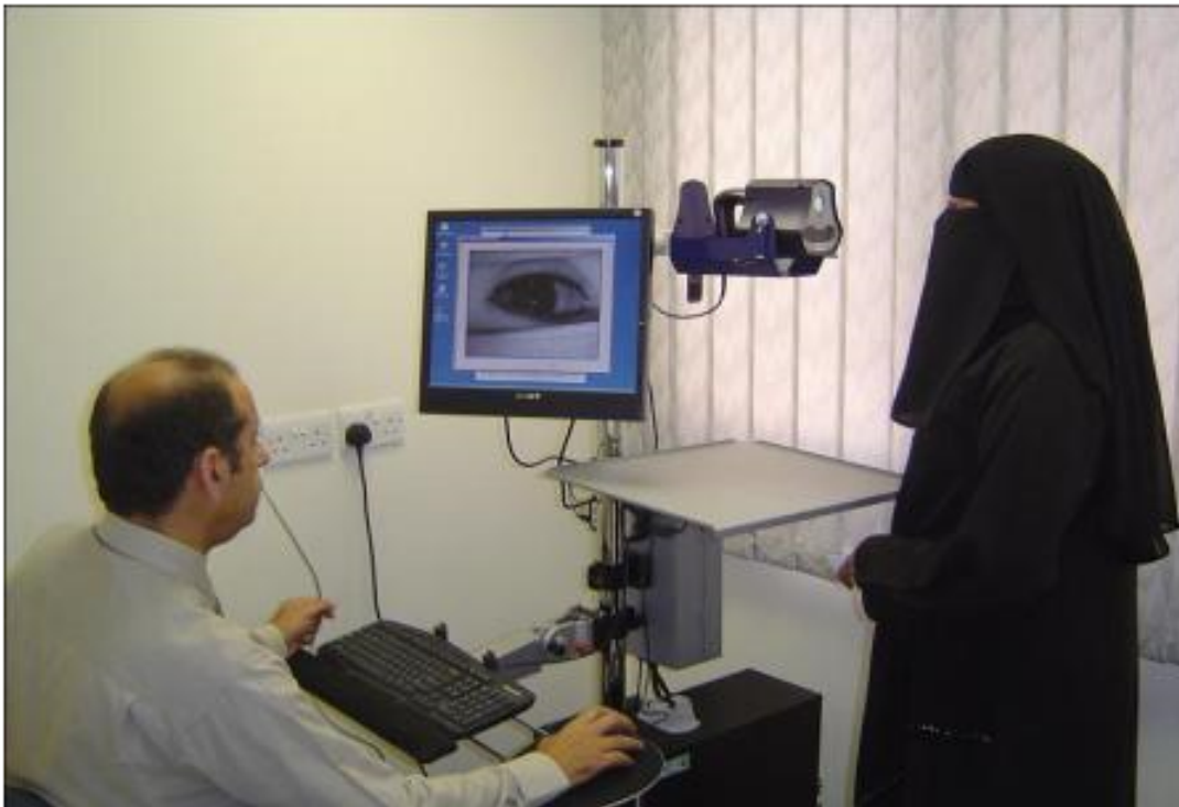
Fig. 2.8 Examples of image acquisition using middle distance device [59]. Adapted with permission from Elsevier. Copyright ©2007 Elsevier Inc.
