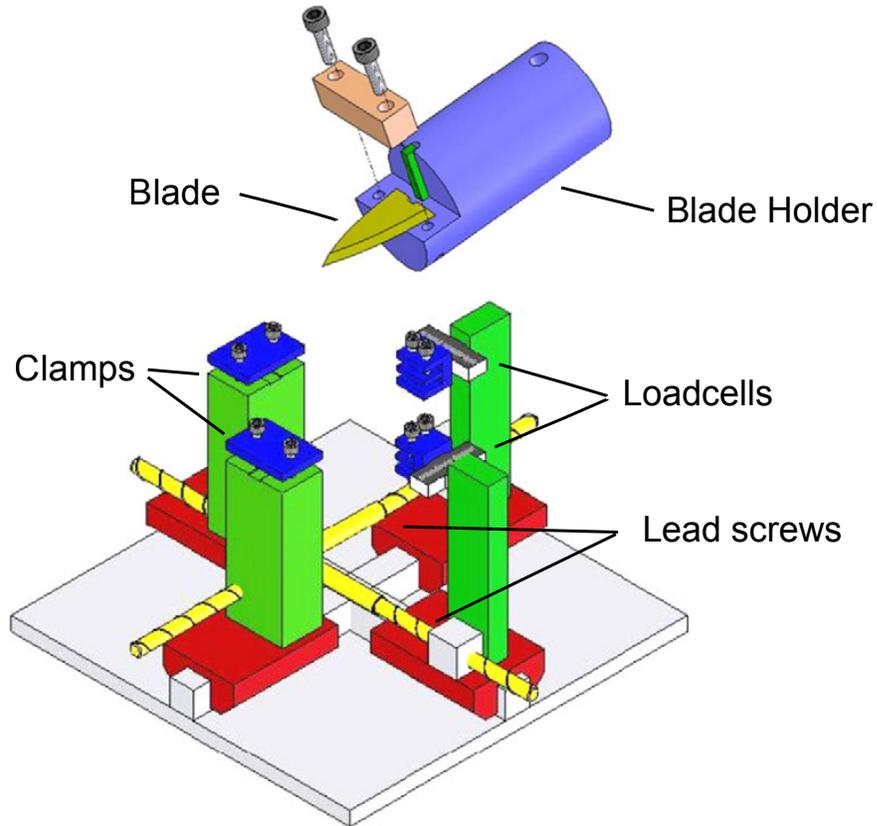
Figure 1: Illustration of biaxial device (Gilchrist et al., 2008).
