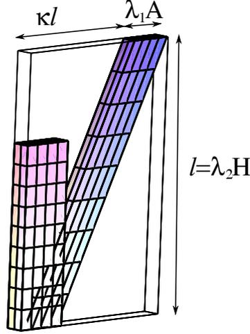
Figure 1: A cuboid of hyperelastic material reinforced with one family of parallel fibers can deform homogeneously when subjected to a tensile force only, as a combination of triaxial stretch (with stretch ratios  $\lambda_i$ ) and simple shear (with amount of shear  $\kappa$ ).
