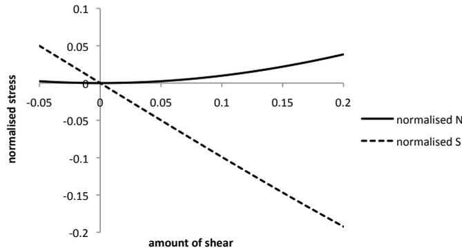
Figure 7: Stresses on inclined faces.
