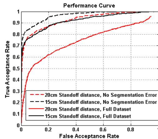
Figure 6. Performance comparison between full image set and image set with improved iris segmentation for 15cm and 20cm stand-off distance.
