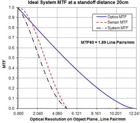
Figure 2. Ideal System Modulation Transfer Function (MTF) plot for 200mm stand-off distance.
