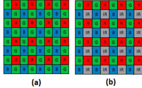
Figure 1. Example for colour filter arrays(CFA) : (a) Bayer CFA, (b) CFA presented in US 8446470 B2. R, G and B represents Red, Green and Blue colour sampling filters respectively. IR represents NIR sampling filter.
