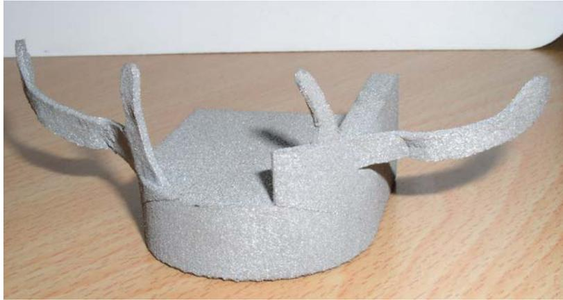
Figure 9: prosthesis model manufactured by solid freeform fabrication of titanium
