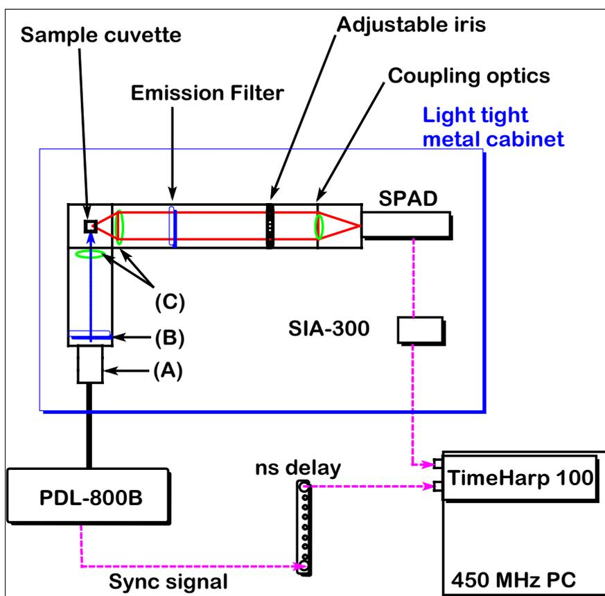
Figure 1: Schematic of fluorescence lifetime measurement apparatus:
