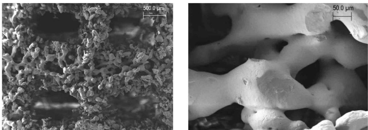
Figure 1 (a) SEM image of designed macropores of the fabricated PCL scaffolds (b) SEM image of microporosity in the designed solid regions of the fabricated PCL scaffolds
