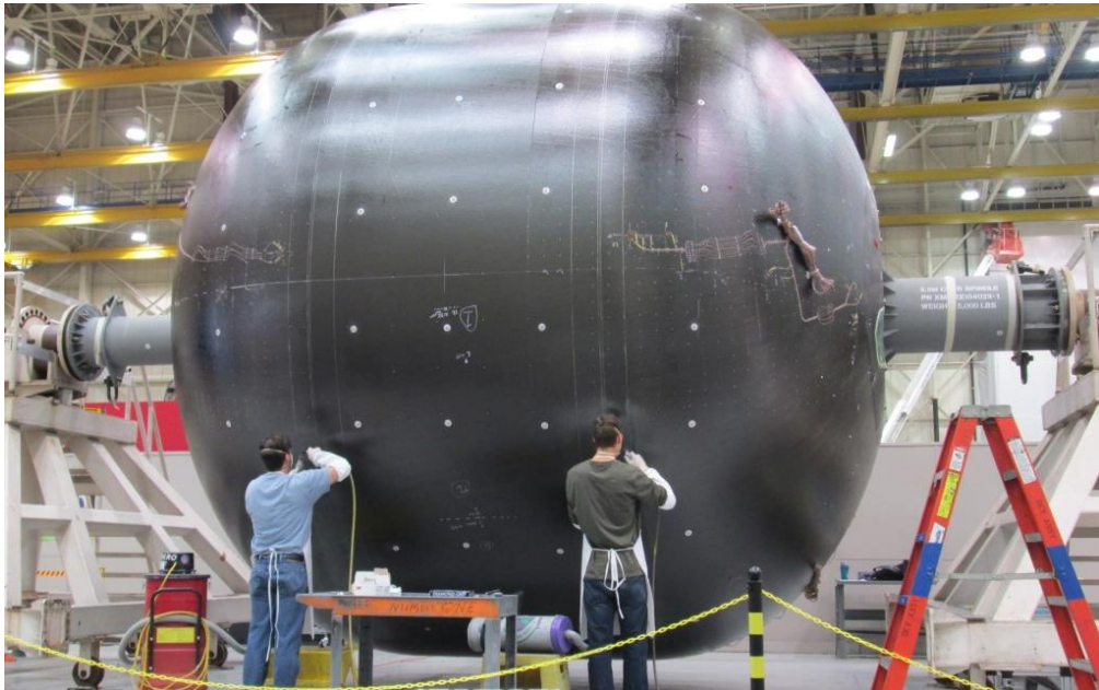
Figure 1.2 A 5.5m diameter composite cryogenic tank prototype under development by Boeing [16]. The tank was manufactured using automated tape placement of thermoset composites.
