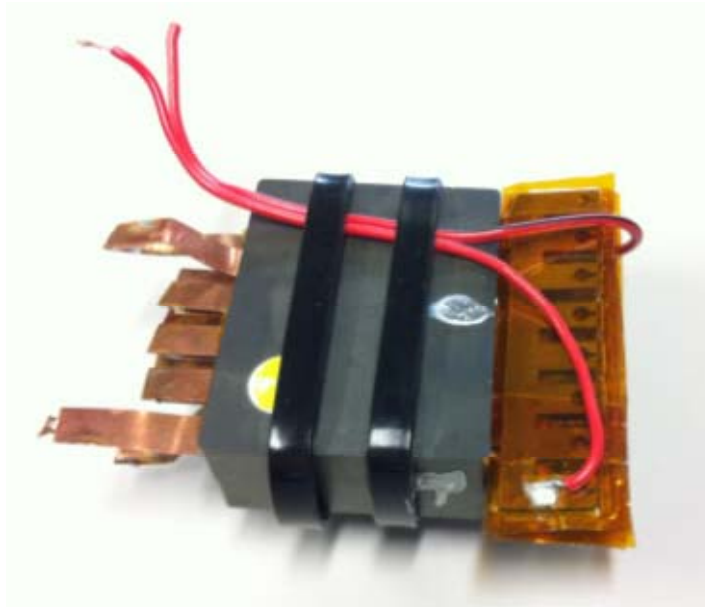
Fig. 6.5 Planar transformer fabricated based on the design results
