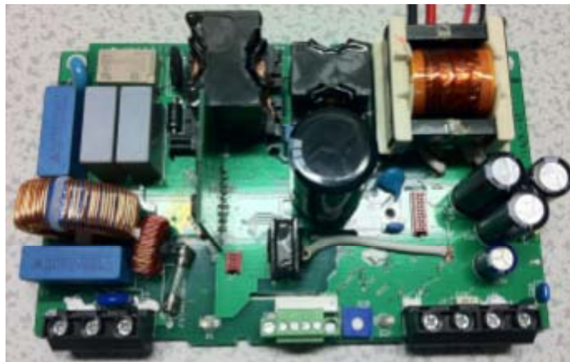
Fig. 2.13 Photo of the tested power supply with the LLC resonant converter
