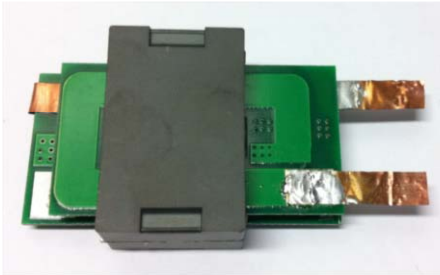
Fig. 5.24 Photo of planar transformer with magnetic shunt (Trans1)
