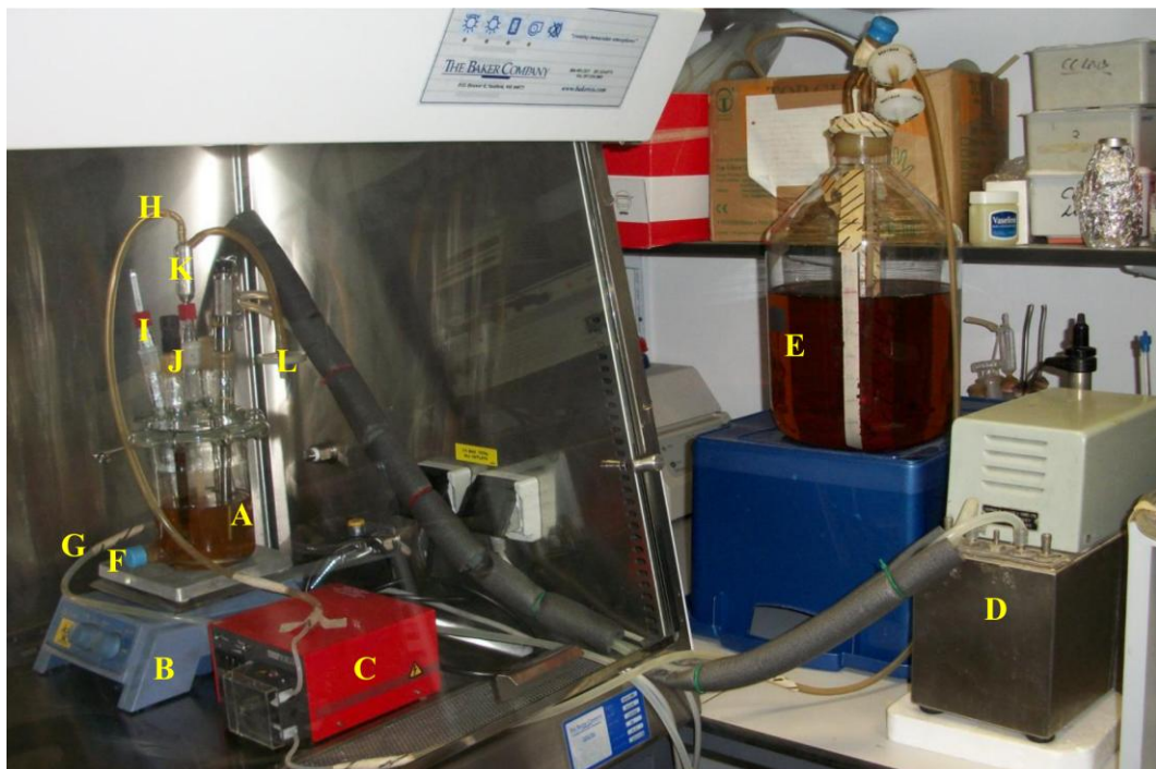
Figure 1.3. The structure of the chemostat used for the long-term disinfectant challenge study. A 545 ml working volume chemostat was used in this study. The fermenter (A) was fed from a 10 litre glass reservoir (E) via a peristaltic pump (C) and feed tubing (H). The constant temperature was maintained by using an internal stainless steel heating coil fed with water from a bath controlled by a water heater (D) and was checked using the thermometer (I). The culture was mixed using magnetic follower on stirrer (B). To make sure that the culture will not be air blocked, the chemostat culture contained medium break (K) and filters (L). The samples for the analysis were collected via sampling port (F). The pH-meter (J) was not used in this study.
