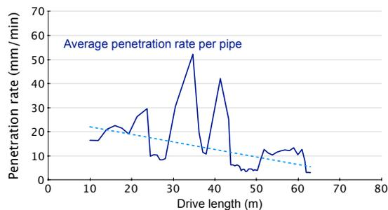
Figure 10 - Penetration rate drive MH 23-22
