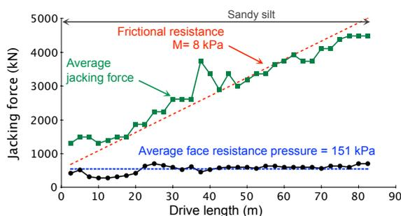
Figure 3 - Jacking force plot MH 2-1
