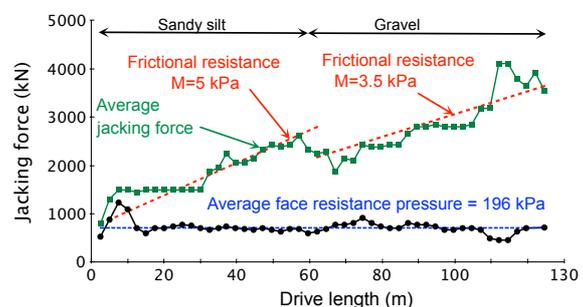
Figure 4 - Jacking force plot MH 2-3
