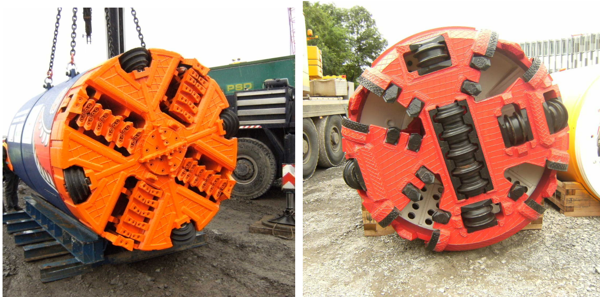
Figure 1 – Mixed ground heads - Iseki TCM 2160 (left) and Herrenknecht AVN1800 (right)
