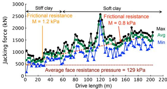
Figure 5 - Jacking force plot for MH 9-11
