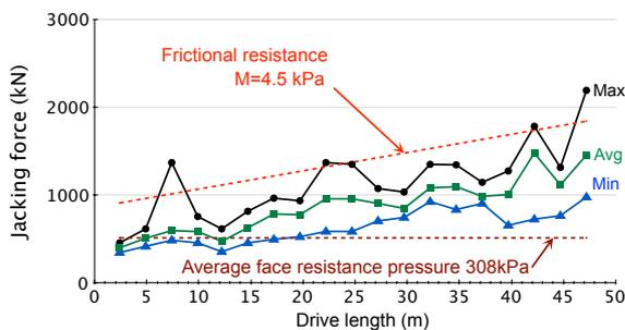
Figure 7 - Jacking force record MH 21-22
