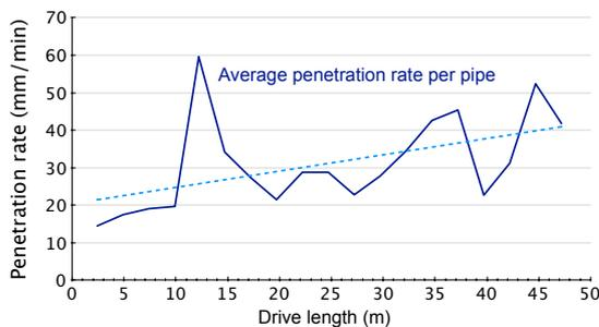
Figure 9 - Penetration rate drive MH 21-22
