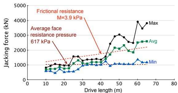
Figure 8 - Jacking force record MH 23-22
