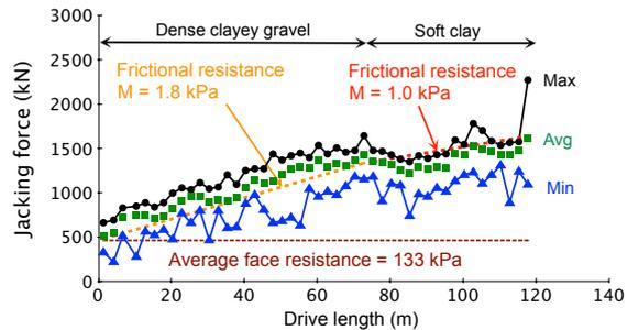
Figure 6 - Jacking force plot for MH 13-11
