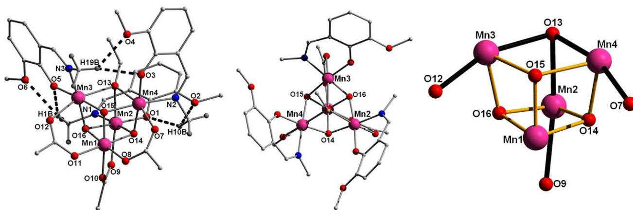
**Figure 6:** (left) Crystal structure of **5**. Dashed lines represent the intra-molecular H-bonds at distances (Å): H19B...O4 = 2.375, H19B...O3 = 2.516, H10B...O2 = 2.547, H10B...O1 = 2.414, H1B...O5 = 2.497, H1B...O6 = 2.660; (centre) View of the pseudo  $C_3$  axis in complex **5**; (right) The cubane core in **5** highlighting (dark lines) the mutually orthogonal Jahn-Teller elongation axes.
