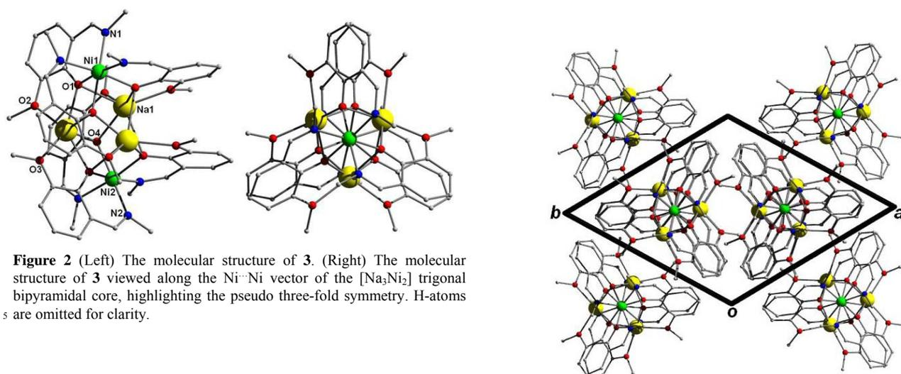
**Figure 2** (Left) The molecular structure of **3**. (Right) The molecular structure of **3** viewed along the Ni-Ni vector of the [Na<sub>3</sub>Ni<sub>2</sub>] trigonal bipyramidal core, highlighting the pseudo three-fold symmetry. H-atoms are omitted for clarity.
