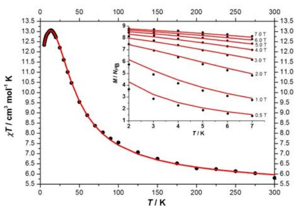
**Fig. 14** Plot of  $\chi_M T$  vs.  $T$  of **6**. Inset: Low temperature magnetisation vs. temperature (at various magnetic fields) plot of **6**. Solid red lines represent best fit to the experimental data.
