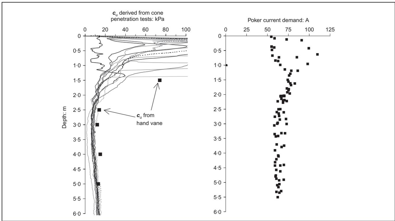
Figure 3. Relationship between undrained shear strength and current demand of poker<sup>5</sup>
