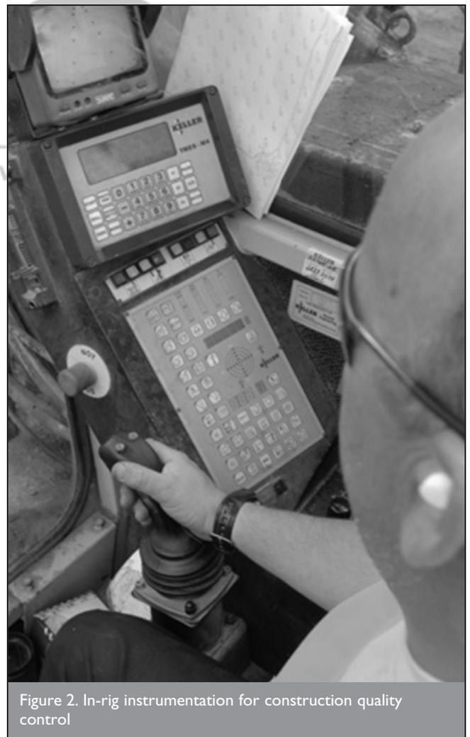
Figure 2. In-rig instrumentation for construction quality control
