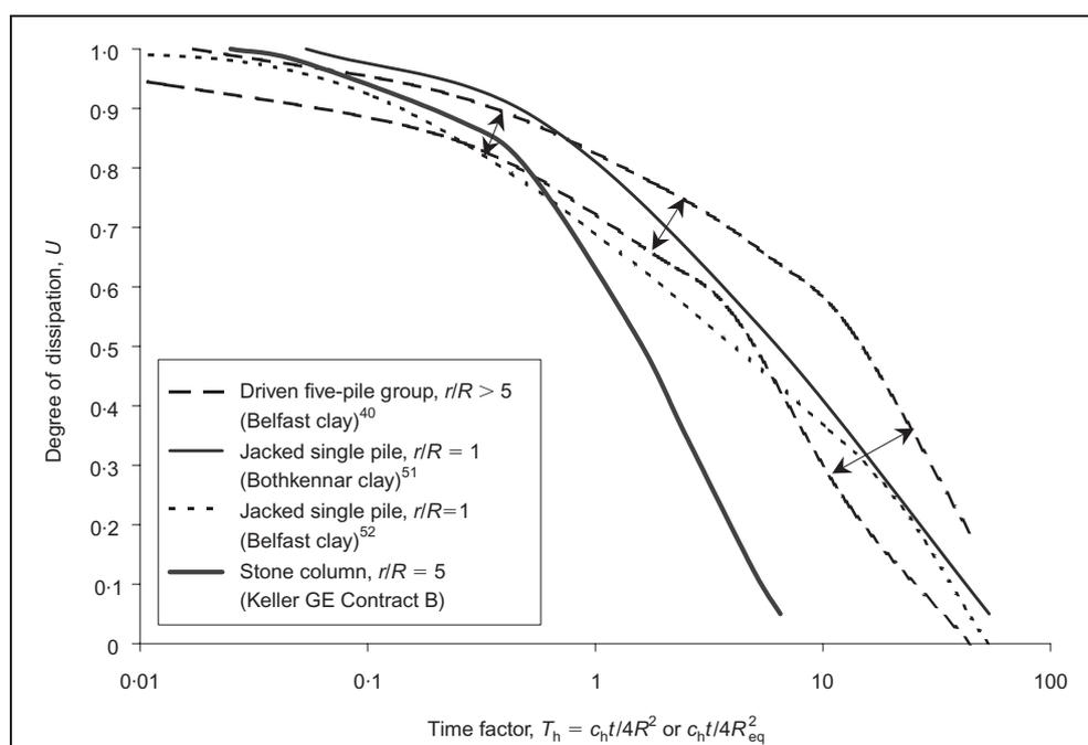
Figure 7. Comparative excess pore pressure dissipation rates for displacement piles and stone columns
