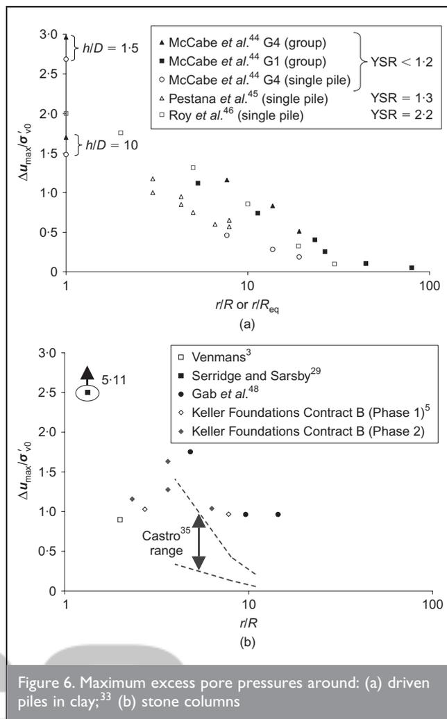
Figure 6. Maximum excess pore pressures around: (a) driven piles in clay,<sup>33</sup> (b) stone columns
