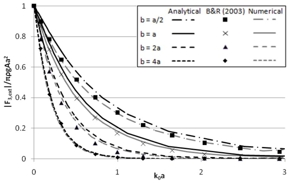
Fig. 7 The normalised heave (or vertical) excitation force, in the frequency domain, as a function of  $k_0 a$ , for various draft-radius ratios compared to Bhatta and Rahman (2003) and to the corresponding numerical CFD analysis.
