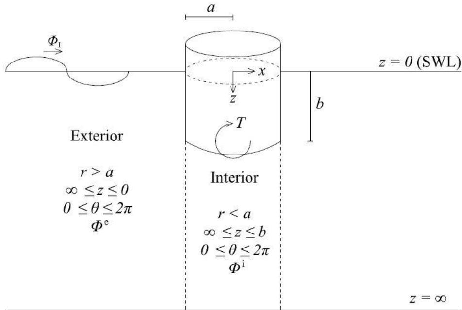
Fig. 1 Definition sketch for the boundary value problem for a truncated vertical cylinder (Finnegan et al., 2011)
