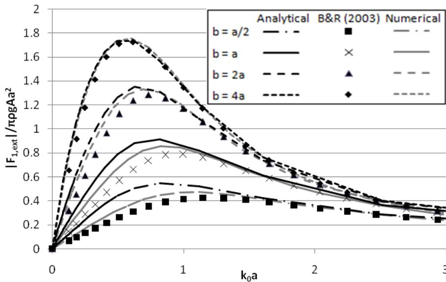
Fig. 6 The normalised surge (or horizontal) excitation force, in the frequency domain, as a function of  $k_0a$ , for various draft-radius ratios compared to Bhatta and Rahman (2003) and to the corresponding numerical CFD analysis
