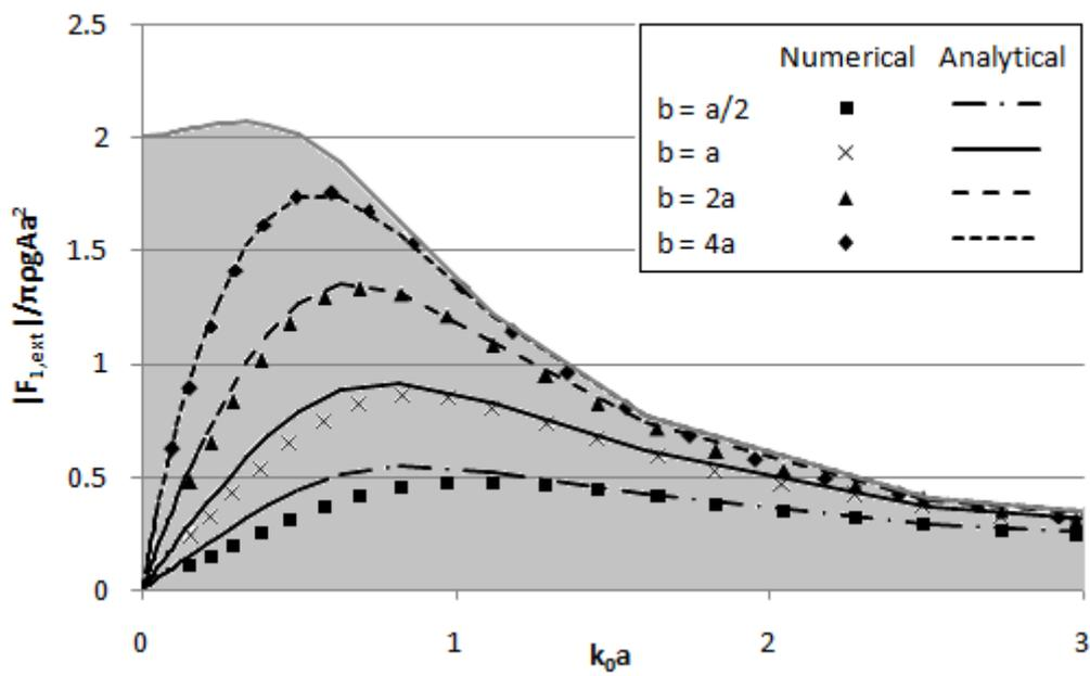
Fig. 2 The normalised surge (or horizontal) excitation force, in the frequency domain, as a function of  $k_0 a$ , for various draft-radius ratios compared to the corresponding numerical CFD analysis
