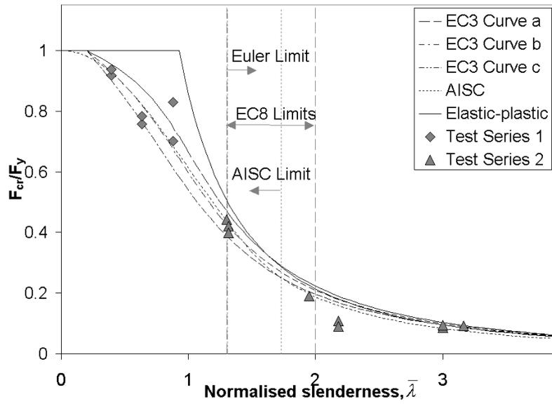
Figure 6. Normalised buckling loads of cyclic specimens.
