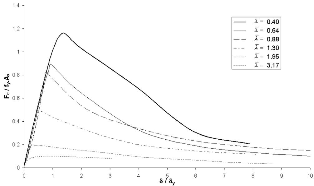
Figure 7. Compression envelope curves for cyclic specimens.
