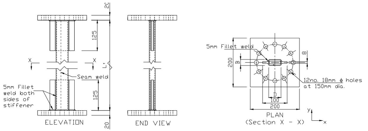
Figure 1. Test specimen.
