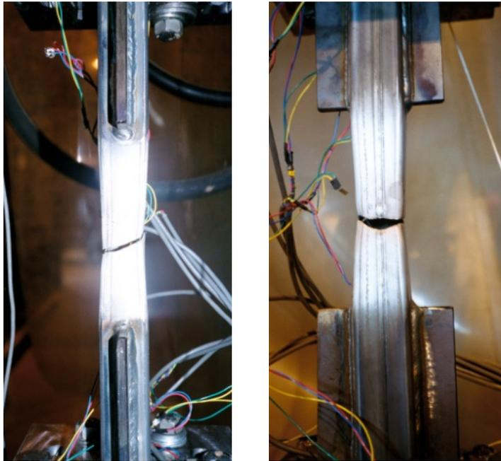
Figure 2: Typical failure of a short specimen in a monotonic tensile test
