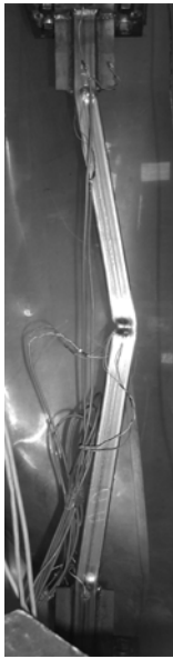
Figure 12 (b). Local and overall buckling of 40x40x2.5SHS hollow specimen CyIS2-40H.
