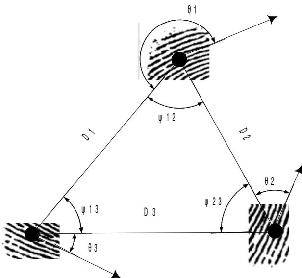
**Fig 2:** Local Triangle Descriptor formed by 3 Minutiae Points
