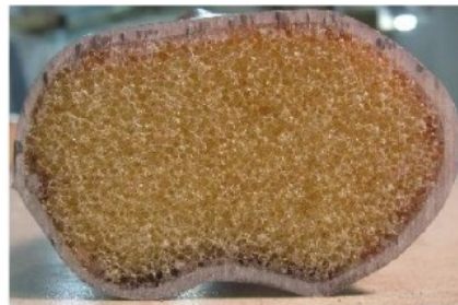
Figure 2-7 The fourth generation composite sawbone tibia used in the present work with a 10 pcf ( \rho = 0.16 \text{ g/cm}^3 ) cellular rigid polyurethane foam core.
