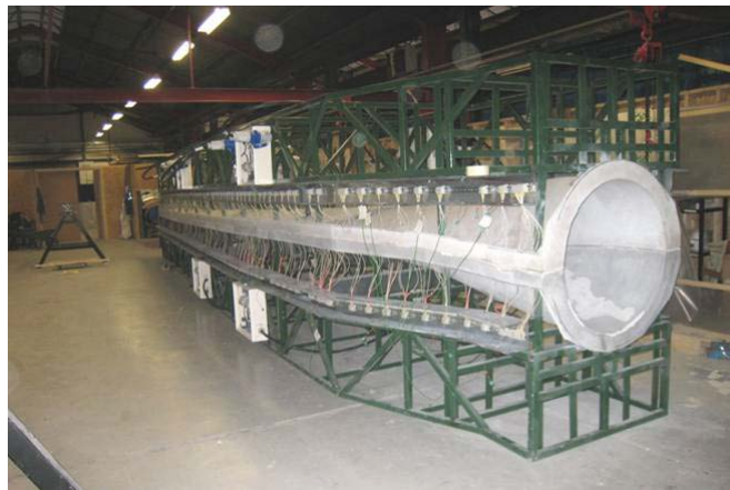
Figure 8. Completed 12.6m wind turbine blade tool
