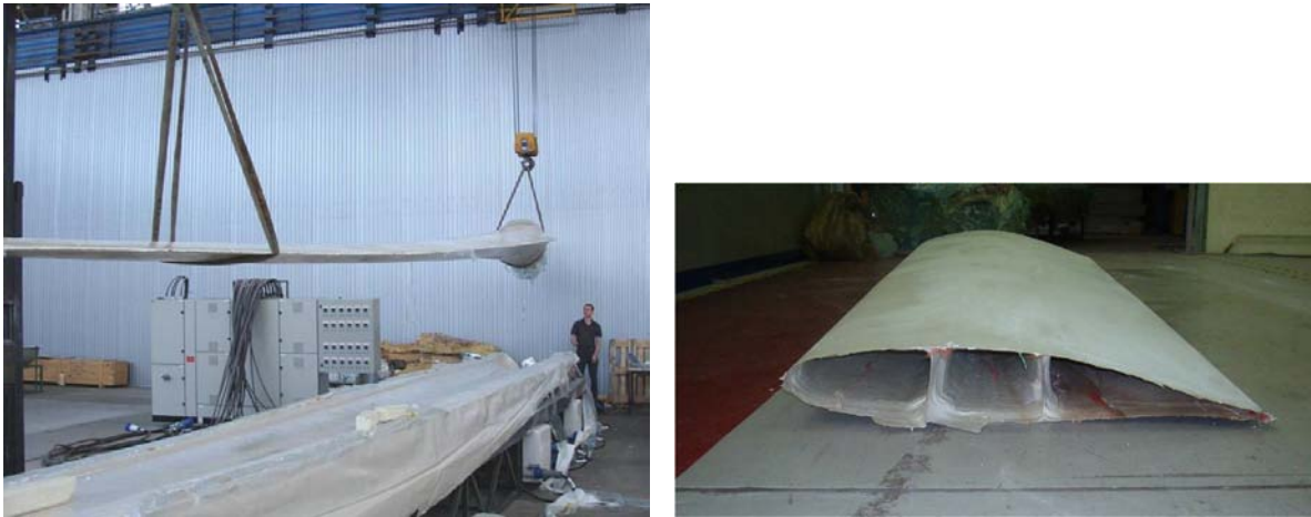
Figure 9. Glass-fibre reinforced PBT thermoplastic wind turbine blade, 12.6 metre length, manufactured at 200°C, (left) removing moulded blade from tool; and (right) a 4.0m moulded section of the blade, showing the spar-cap and shear-webs moulded in a “one-shot” process.
