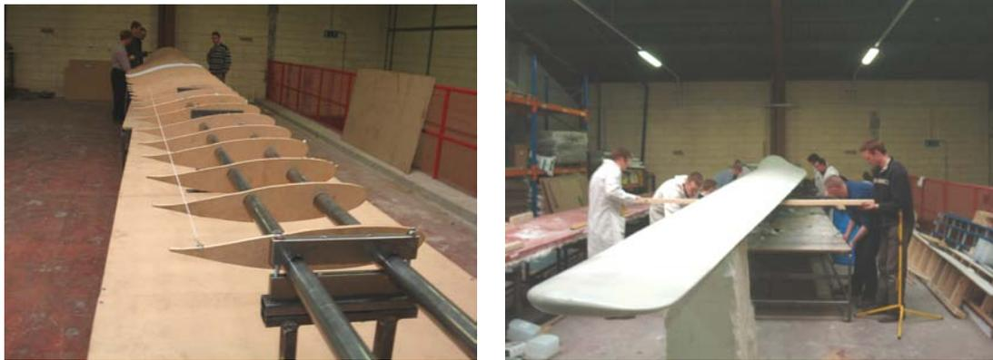
Figure 7. Construction of 12.6m wind turbine blade pattern
