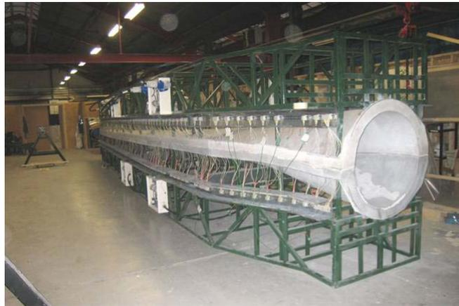
Figure 8. Completed 12.6m wind turbine blade tool
