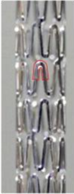
Figure 6-1: An example of a cardiovascular stent architecture consisting of a series of repeating interconnected unit cells (highlighted), where each unit cell consists of an arch connected to straight struts (Parry and McGarry, 2012).
