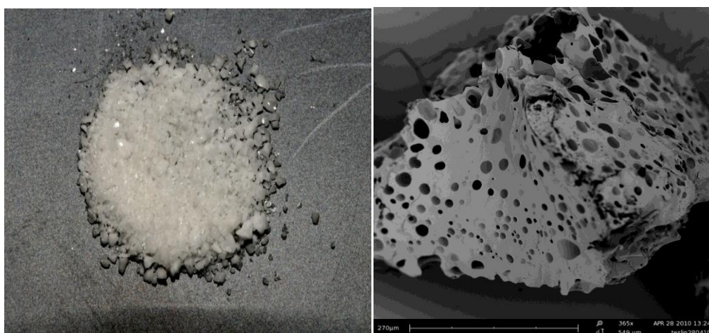
FIGURE 4.04: Photograph (left) and SEM image (right; scale bar is 270 \mu\text{m} ) of purified poly(NIPAM) obtained at 71% conversion.
