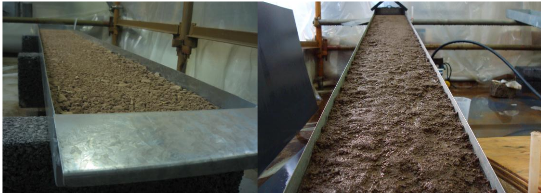
Figure 3.4 Soil in laboratory flume before and after rainfall simulation.
