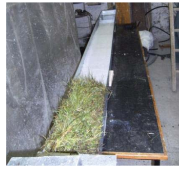
View of runoff box with one sod
