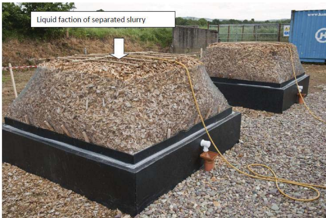
Figure 2.12 Pilot scale wood chip filter used to treat the liquid portion of pig slurry following separation (Carney et al., 2011)
