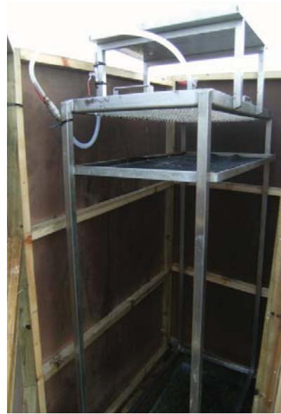
View of rainfall simulator before rainfall starts
