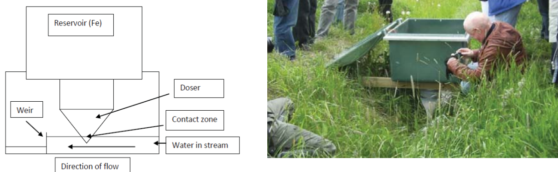
Figure 2.11 Schematic and photo of ferric-sulphate doser in operation in Jokioinen, Finland (Narvanen et al., 2008)
