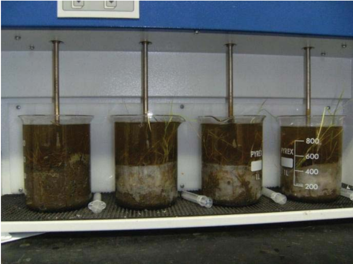
Figure 3.1 Beakers placed in flocculator during agitator test
