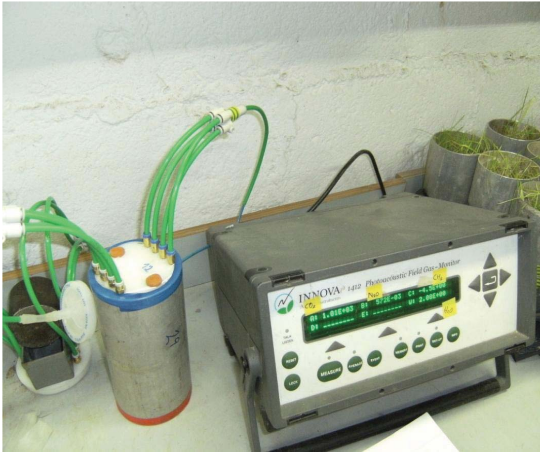
Figure 5.4 Photograph of PAA during carbon dioxide, methane and nitrous oxide measuring period
