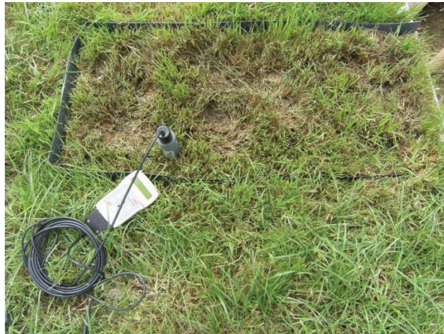
Figure 6.5 Photo of the measurement of volumetric water content of soil using time domain reflectometry
