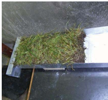
Soil samples placed in flume starting at lower end
