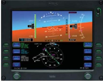
Figure 1. The Avidyne primary flight display (PFD). The same display was used for training in the flight simulator and in the transfer aircraft.
