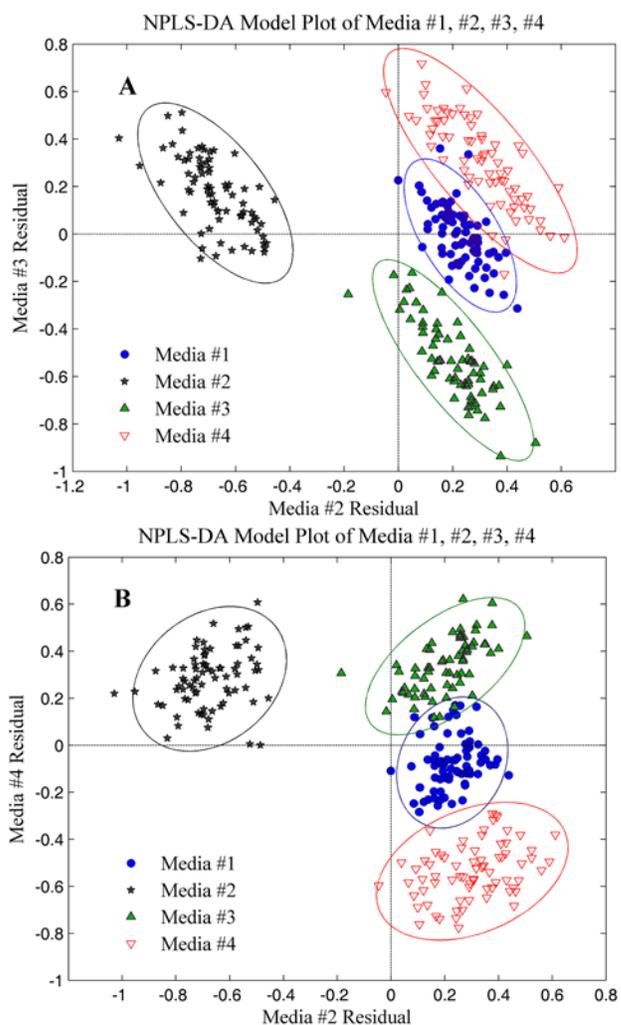
**Figure 3:** Overview of the NPLS-DA model (five LVs used on the Rayleigh scattering corrected fluorescence EEM data) on the 290 measurements of four types of media samples (Table 1). A solid ellipse specifies a distribution of normal measurements for each class. The plots show that the media composition (as measured by the EEM spectra) is changing subtly on prolonged storage. [More detail in supplementary information, figure S-8]
