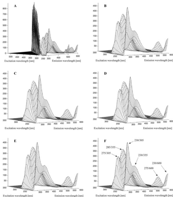
**Figure 1:** EEM landscapes of representative samples of feed medias#1-4. (A) Original Media#1 spectrum. Rayleigh corrected spectra of Medias: #1 (B), #2 (C), #3 (D), and #4 (E). (F) Rayleigh corrected Media#1 sample showing local intensity maxima, arrows point to local excitation/emission peaks (Table 1).
