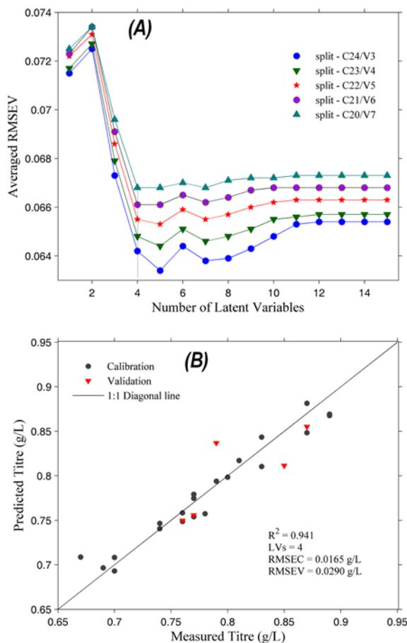
**Figure 4:** (A) Results of cross-validation for latent variables selection to yield appropriate NPLS model for the averaged EEM data of 27 Media#1 samples; (B) NPLS model for the correlation between Media#1 EEM data and end protein product yield. Calibration model used a set of 22 randomly selected averaged Media#1 EEM spectra and validated with the 5 remaining EEM spectra.
