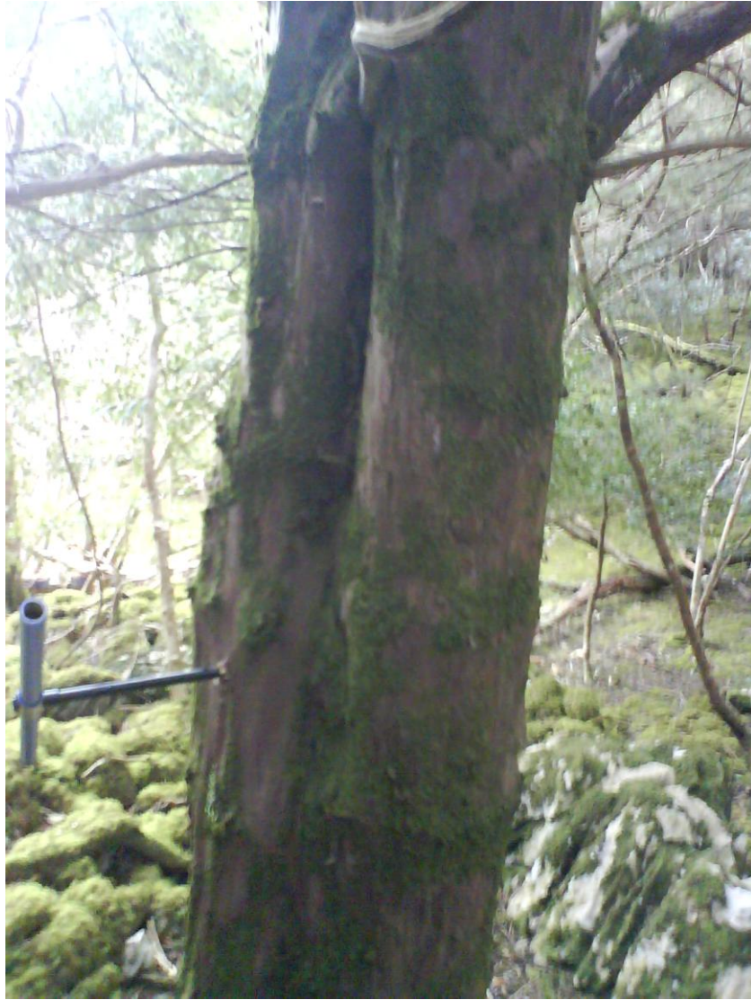
Figure B1: T. baccata tree in Reenadinna Wood, Killarney National Park, with 5.15 mm two-thread Haglöf increment borer.
