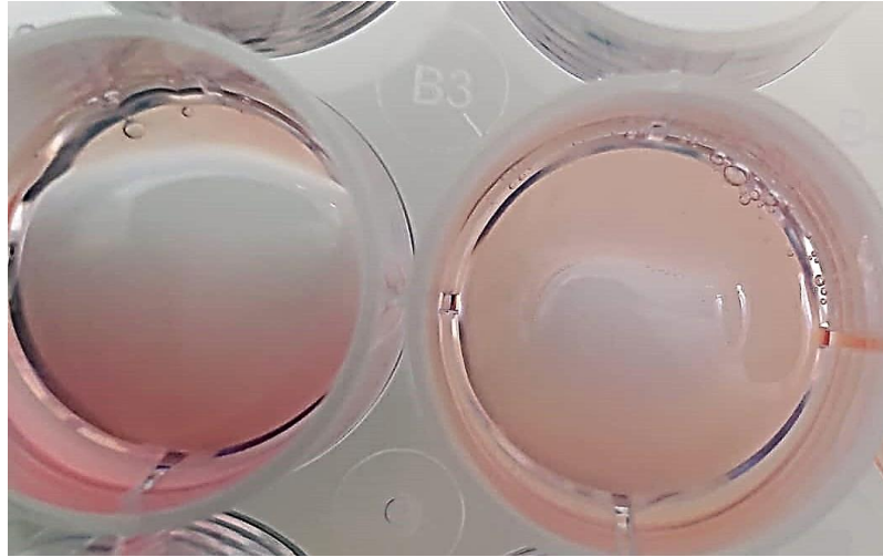
Figure 3.9. Broken collagen I hydrogels after ablation. Left hydrogel was treated with 750V and right hydrogel was treated with 500 V.
