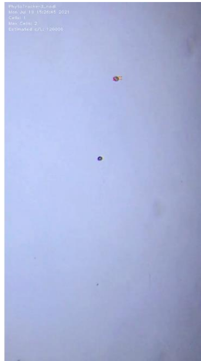
Figure 34 Screen grab from a HABscope video demonstrating two cells identified using the neural network programme trained to recognise Karenia spp. cells
