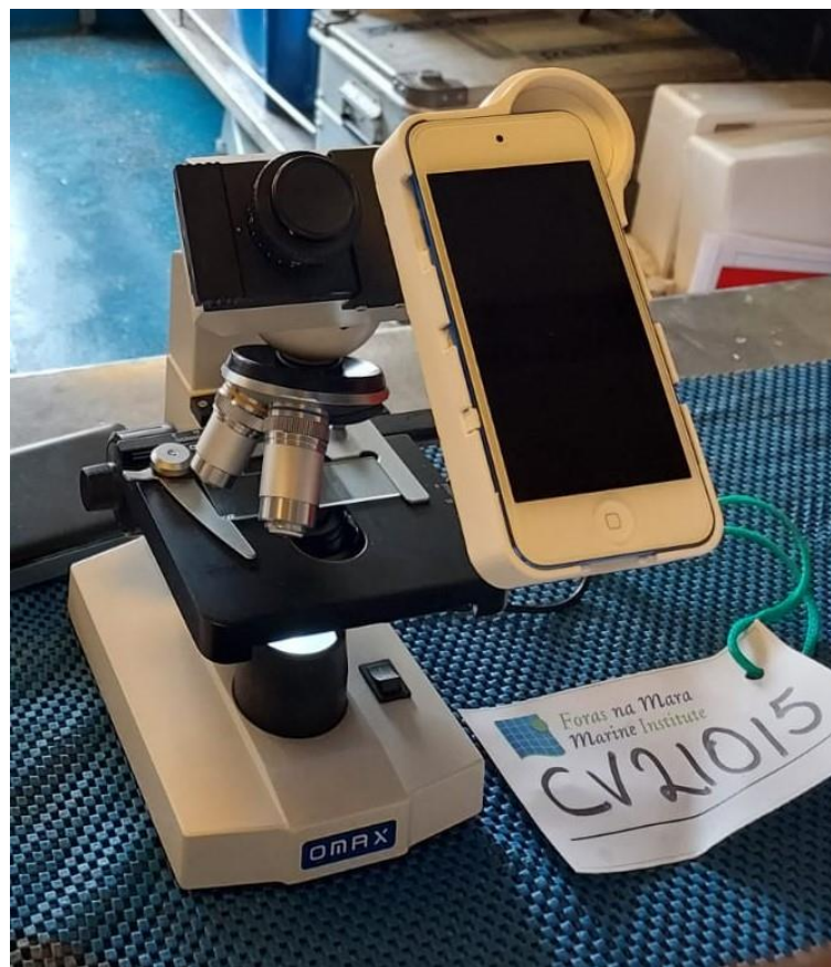
Figure 32 HABscope set up on research survey CV21015
