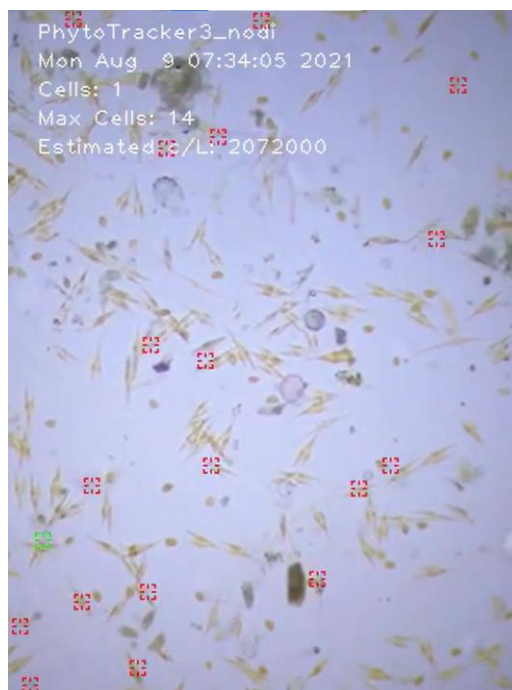
Figure 36 Screen grab from the HABscope to illustrate a mixed assemblage of phytoplankton species and the neural network technology identifying Karenia spp. amongst other species
