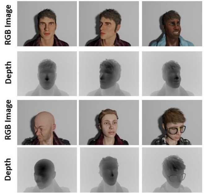
Fig. 9. Sample images of virtual human faces and their ground truth depth (scaled to visualize) with different head pose
