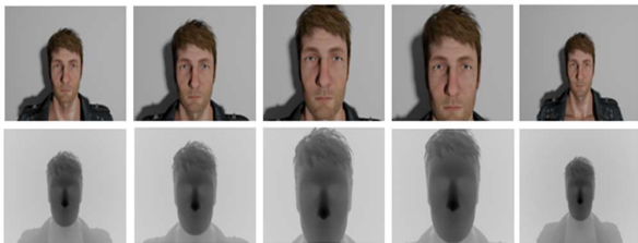
Fig. 6. A facial model with ground truth depth captured at the different camera position.
